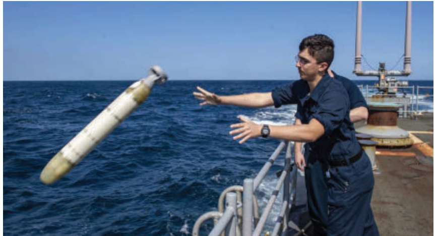
Researchers are using the MK 39 Mod 2 expendable mobile antisubmarine warfare (ASW) training targets (EMATT) from Lockheed Martin Sippican Inc. in Marion, Mass., for swarming UUV development.
